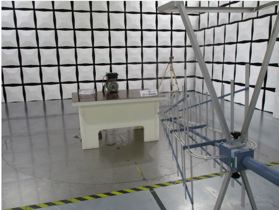
Photograph 3: Radiated emission measurements test set-up Front side view
