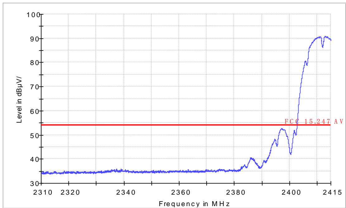
FCC Electric Field Strength 2.4GHz Bandedge-AV
