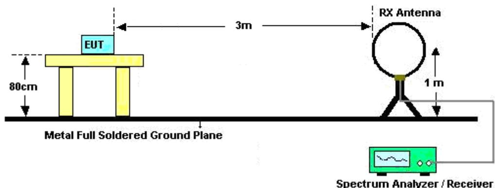
For radiated emissions from 30MHz to 1GHz
