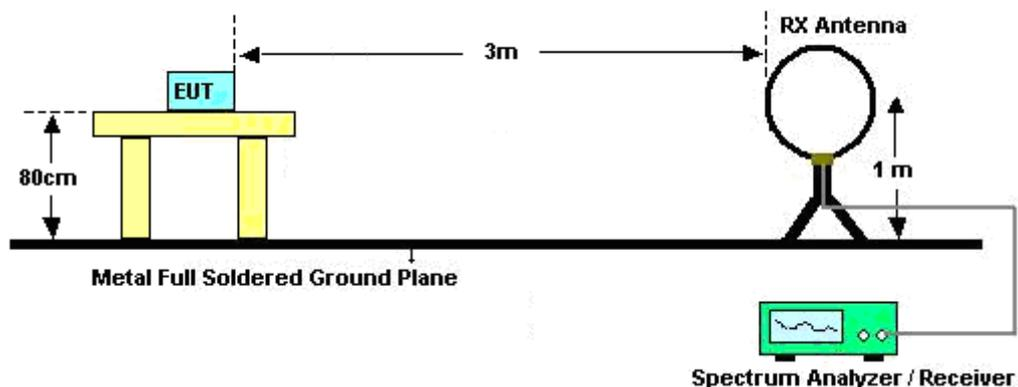
For radiated emissions from 30MHz to 1GHz
