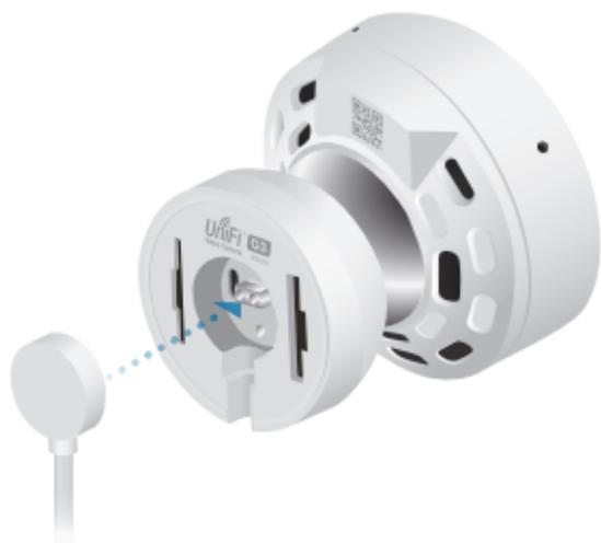
4. Attach the camera and *Magnetic Base* to the mount. If the power cord feeds through the *Wall Mount*, rotate the *Magnetic Base* to align the cord with the notch on the *Wall Mount*. Go to *Connecting the Power*.
