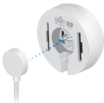
3. Attach the *Magnetic Base* of the camera to the *Instant PoE Mount* by pressing it over the two notches and sliding it down.
