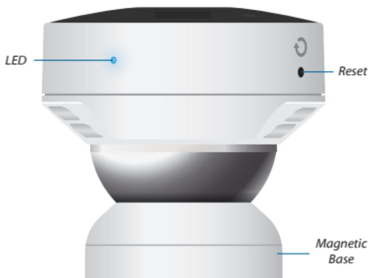
**LED** The LED will flash blue during bootup. When the camera is ready to connect to the Wi-Fi network, the LED pattern will flash two times accompanied by two beep tones. Once connected to the network, the LED will glow a breathing pattern.
