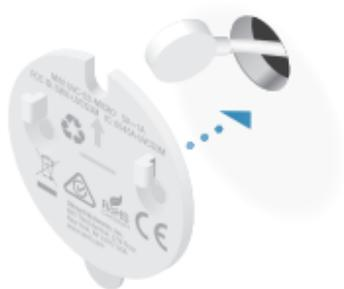
2. Remove the tab from the notch and attach the *Wall Mount* using the adhesive side.
