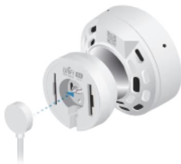
3. Attach the *Magnetic Base* of the camera to the *Table Stand* by pressing it over the two notches and sliding it down.
