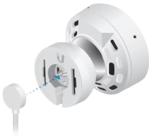
4. Attach the camera and *Magnetic Base* to the mount. If the power cord feeds through the *Wall Mount*, rotate the *Magnetic Base* so the cord aligns with the notch on the *Wall Mount*. Go to *Connecting the Power*.
