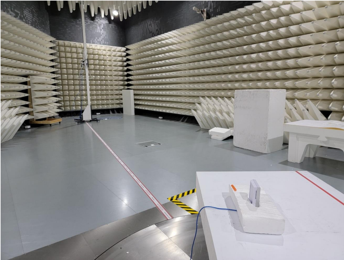
Photograph 1: View Test Set Up Radiated Emissions 30 – 1000 MHz
