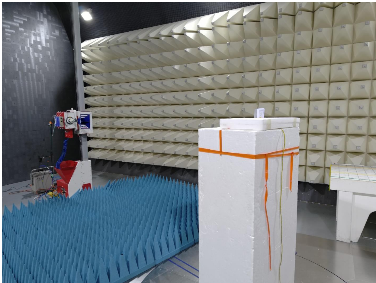
Photograph 2: View Test Set Up Radiated Emissions 1 – 17 GHz
