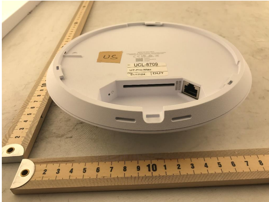
Photograph 3: Back View of DUT Showing RJ45 Port
