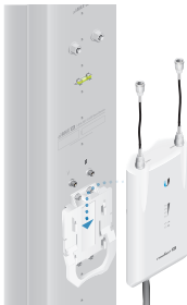
Mounting on a Sector Antenna
