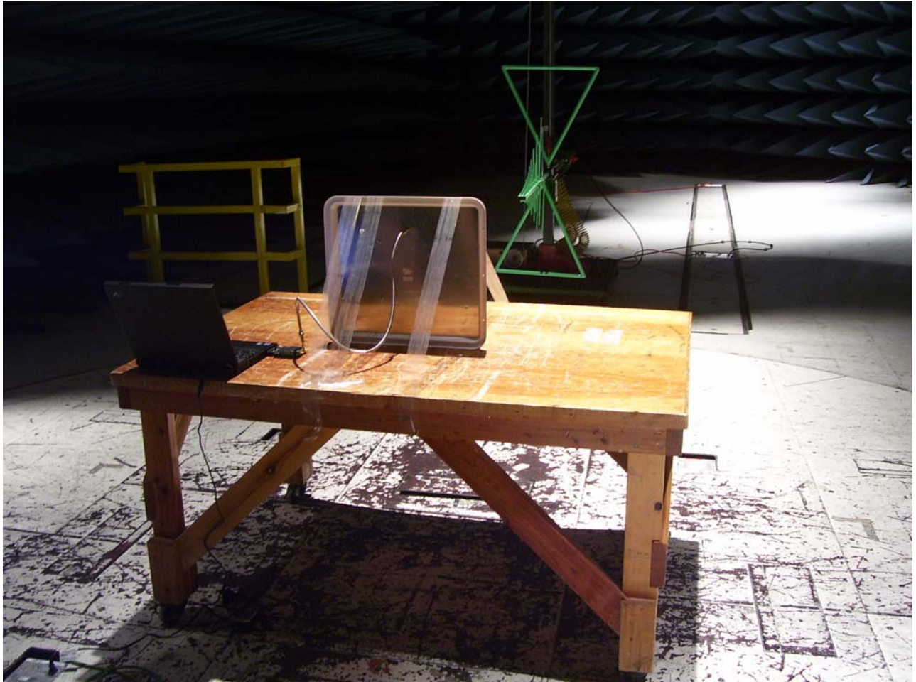
Photograph 4. Radiated Emission Test Setup 30 MHz - 1 GHz
