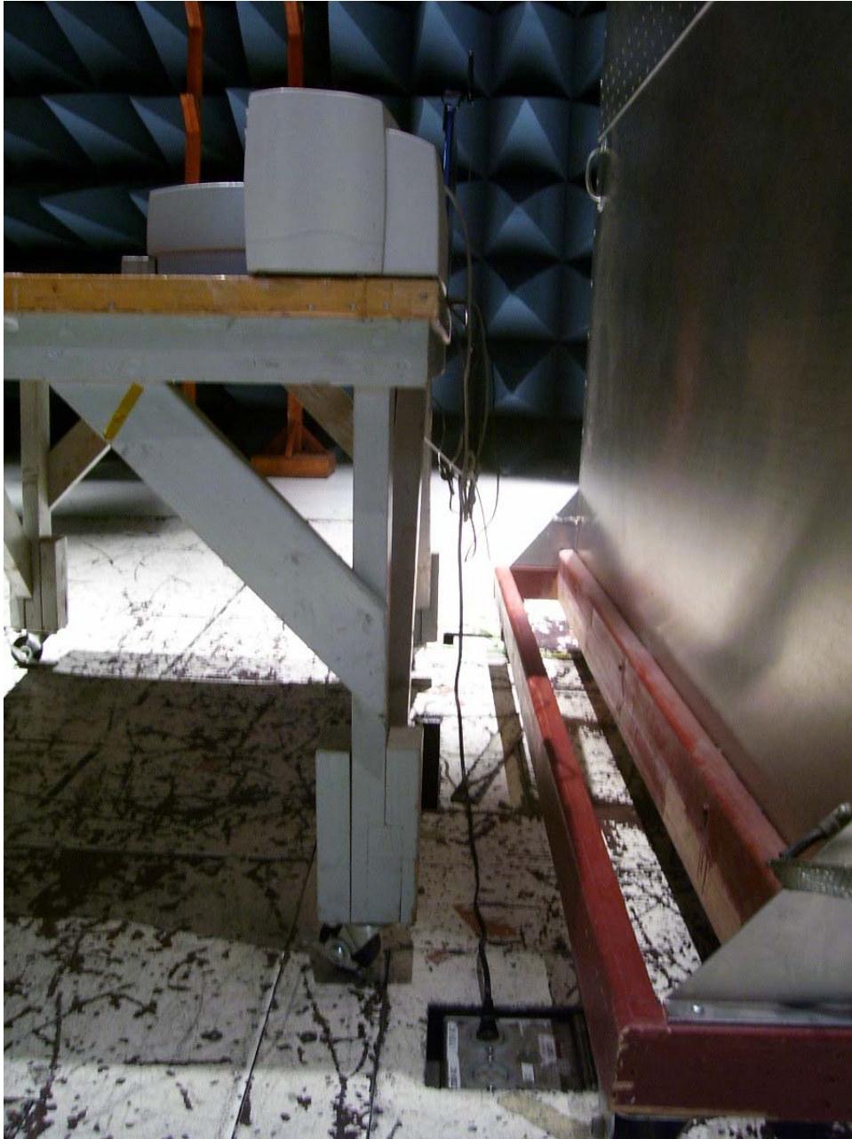
Photograph 3. Conducted Emissions Test Setup – Rear View
