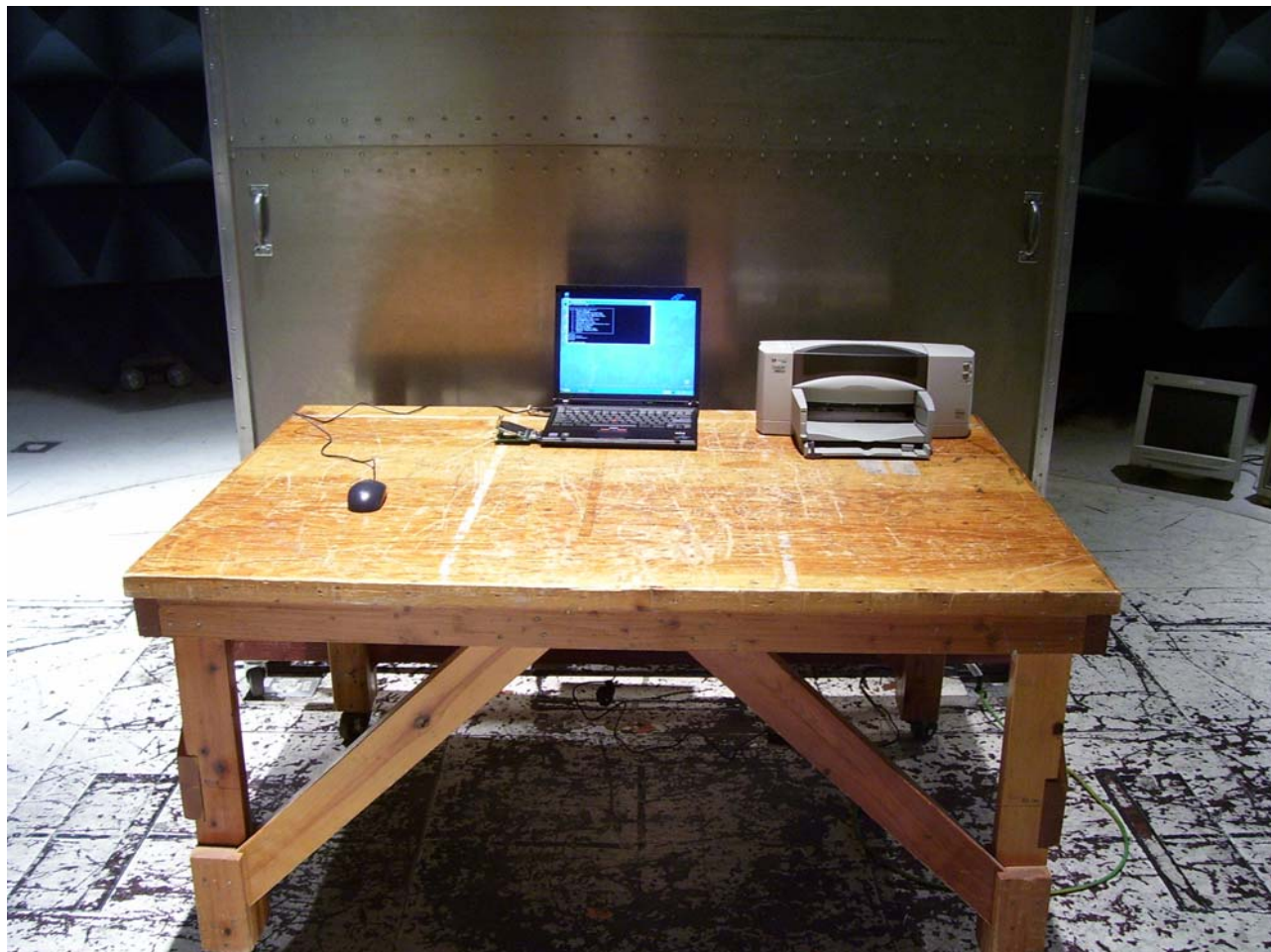
Photograph 2. Conducted Emissions Test Setup
