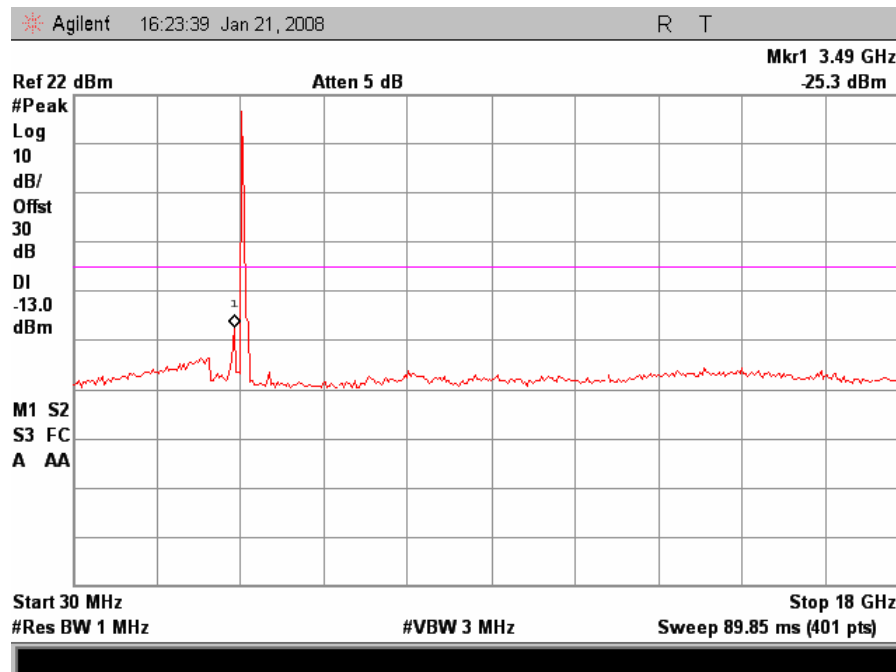
Plot 32. Conducted Spurious Emissions 10 MHz Low Ch (30 MHz - 18GHz)
