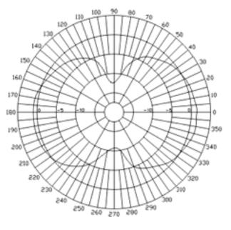
Model Hyperliniktech HG2403RD-RSF Type: Dipole Gain: 3dBi
