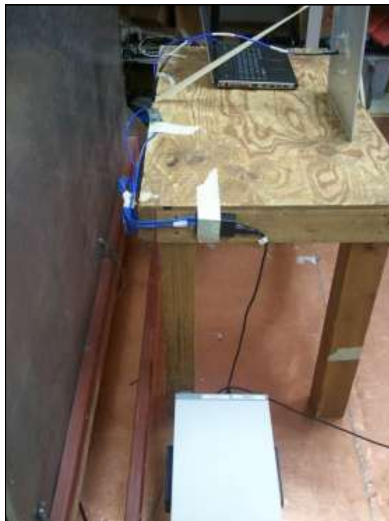
Photograph 8. Conducted Emissions, 15.207(a), Test Setup, Side View
