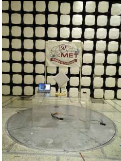
Photograph 4. Radiated Emissions, Test Setup
