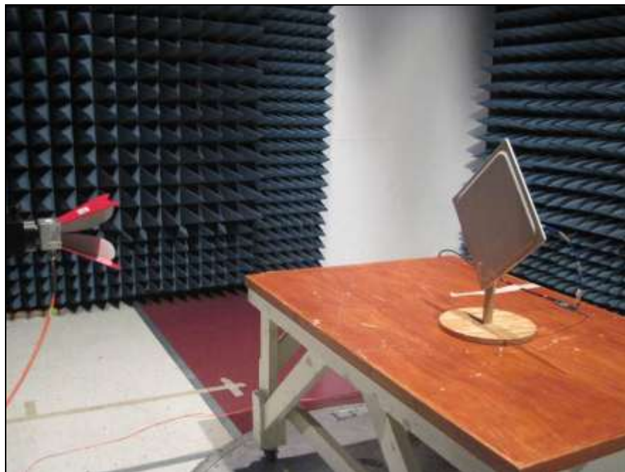
Photograph 10. Radiated Spurious Emissions, Test Setup, 1 GHz – 18 GHz
