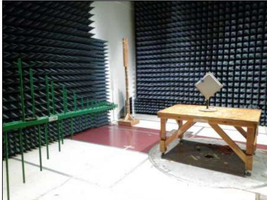
Photograph 9. Radiated Spurious Emissions, Test Setup, 30 MHz – 1 GHz
