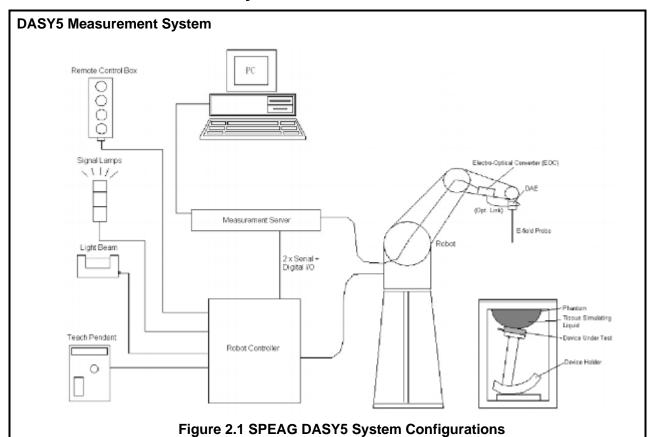
The DASY5 system for performance compliance tests is illustrated above graphically. This
