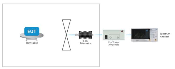
Figure 3: Radiated Emissions Test
