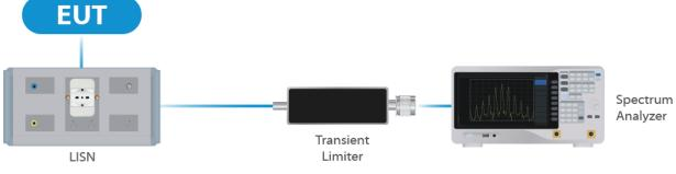
**Figure 1: Conducted Emissions Test**
