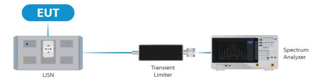
**Figure 1: Conducted Emissions Test**
