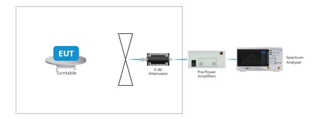
Figure 4: Radiated Emissions Test
