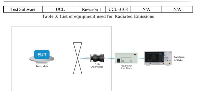
Figure 4: Radiated Emissions Test
