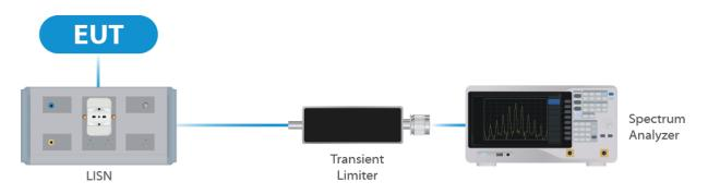
**Figure 1: Conducted Emissions Test**
