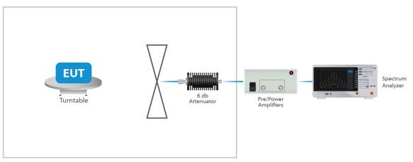
**Figure 2: Radiated Emissions Test**
