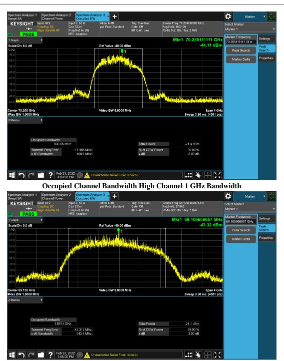
Occupied Channel Bandwidth High Channel 2 GHz Bandwidth
