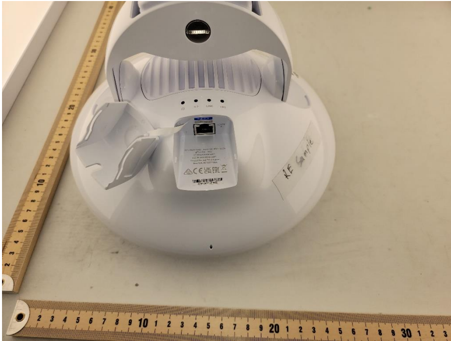
Photograph 3: Back View of DUT Cover Removed Showing RF45 Jack
