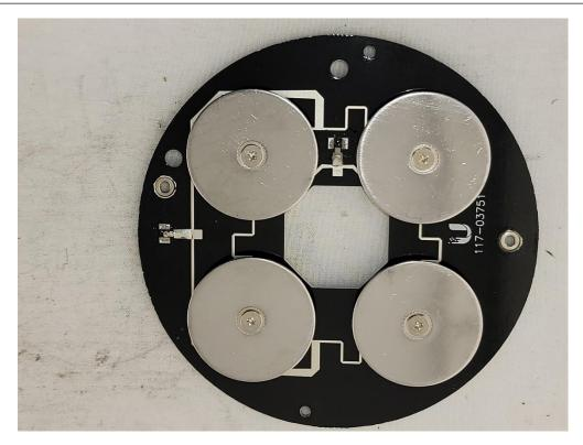
Photograph 8: Front View of the 5GHz Antenna
