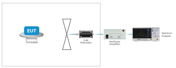
Figure 3: Radiated Emissions Test
