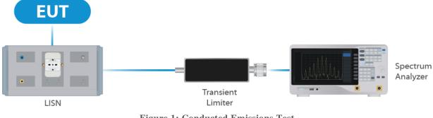
**Figure 1: Conducted Emissions Test**
