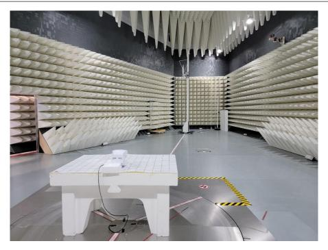
Photograph 1: View Test Set Up Radiated Emissions 30 – 1000 MHz
