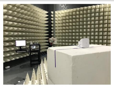
Photograph 3: View Test Set Up Radiated Emissions 17 – 40 GHz
