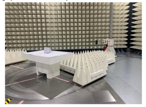
Photograph 2: View Test Set Up Radiated Emissions 1 – 17 GHz
