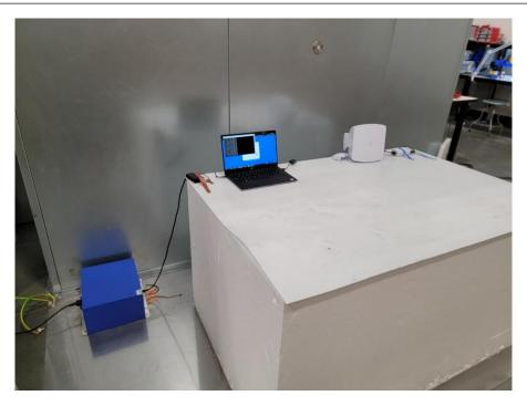
Photograph 5: Front View Test Set Up AC Mains Conducted Emissions
