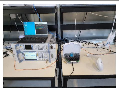
Photograph 7: Test Set Up DFS Conducted
