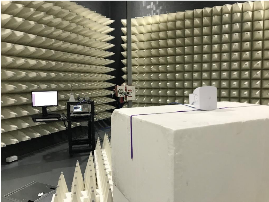
Photograph 3: View Test Set Up Radiated Emissions 17 - 40 GHz
