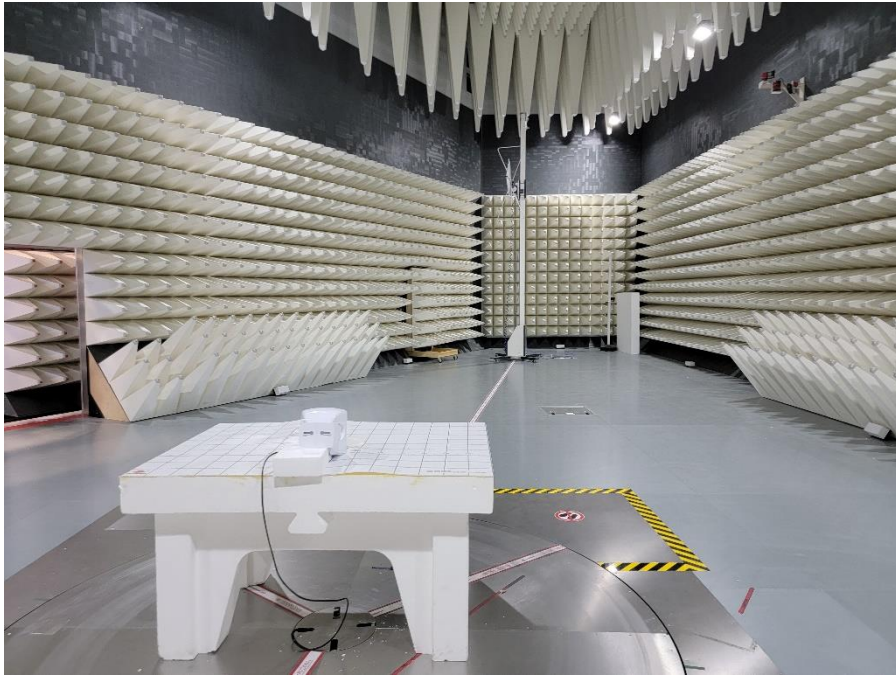
Photograph 1: View Test Set Up Radiated Emissions 30 – 1000 MHz
