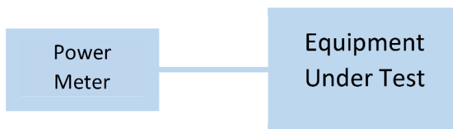
Figure 3: Output Power Measurement
