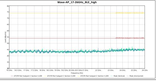
\* No significant emissions were observed in either Vertical or Horizontal Polarity
