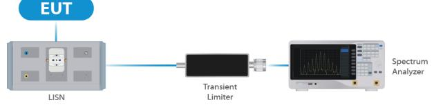
**Figure 1: Conducted Emissions Test**
