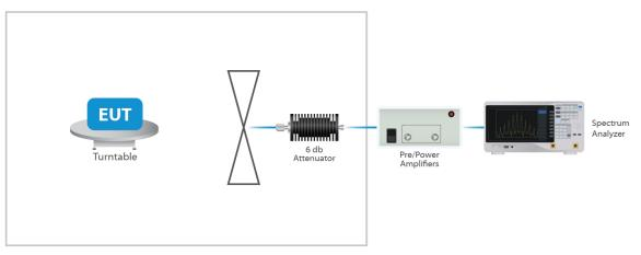
Figure 3: Radiated Emissions Test
