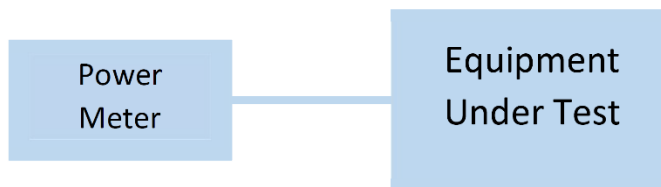
Figure 3: Output Power Measurement
