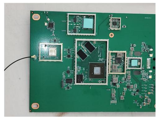
**Photograph 5: PCB Bottom (Shields Removed)**
