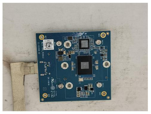
Photograph 7: 60GHz Antenna and module Bottom
