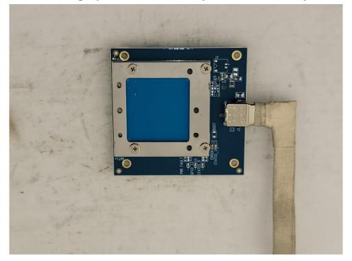
Photograph 6: 60GHz Antenna and module Top
