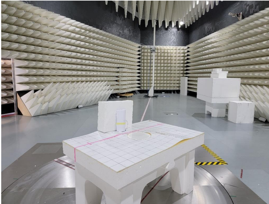
Photograph 1: View Test Set Up Radiated Emissions 30 – 1000 MHz
