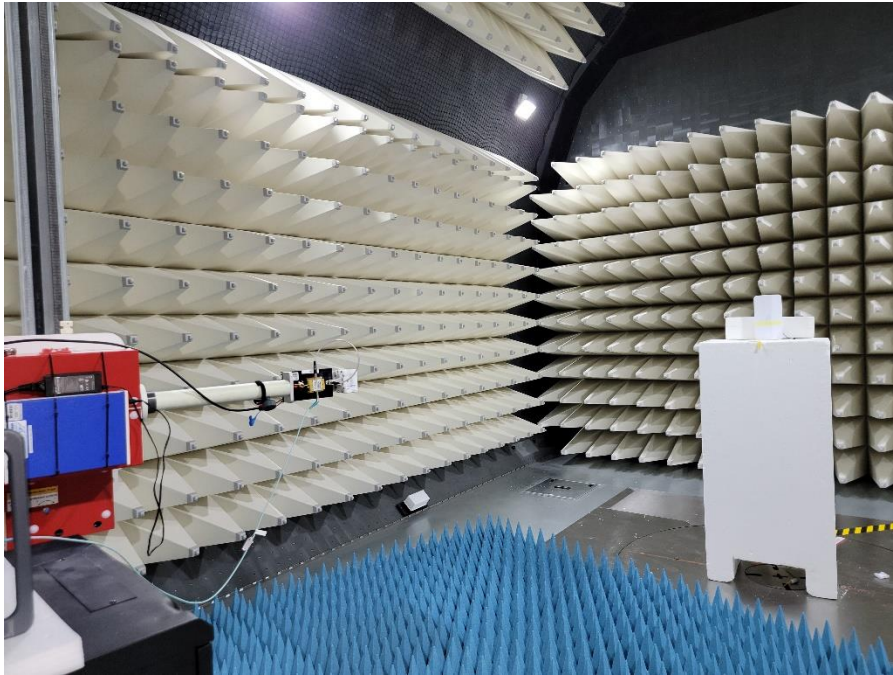
Photograph 3: View Test Set Up Radiated Emissions 17 – 40 GHz
