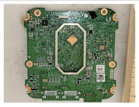
**Photograph 5: PCB EMI Shield Removed**
