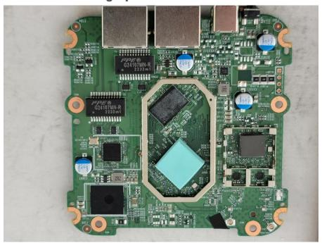
Photograph 4: PCB EMI Shields removed
