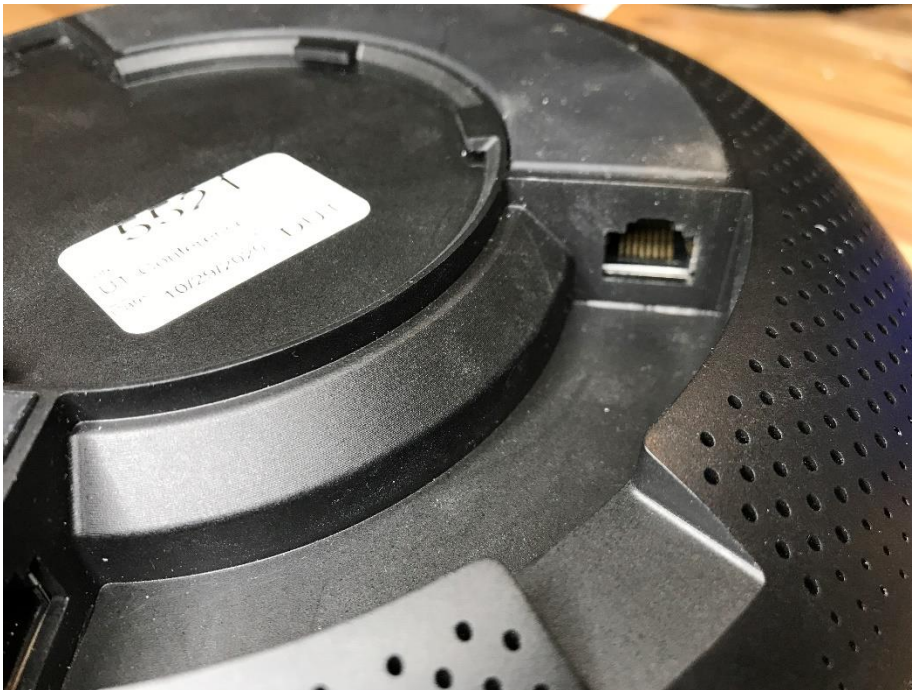
Photograph 8: Close Up Of POE Out Port
