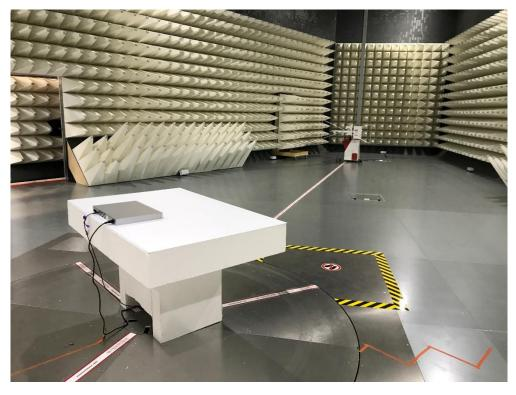
Photograph 1: Side View Test Set Up 30 – 1000 MHz
