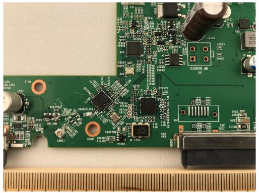
Photograph 4: Top View of Bluetooth Transmitter Circuit Board
