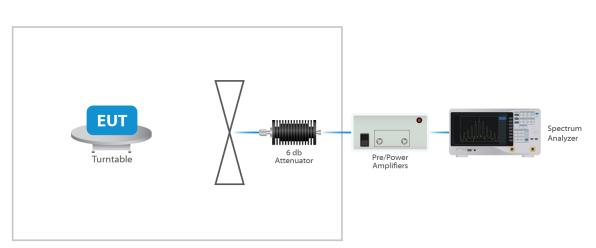
Figure 3: Radiated Emissions Test
