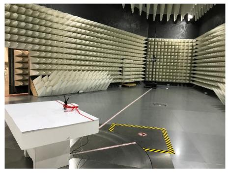
Photograph 1: Test Set Up Radiated Emissions 30 – 1000 MHz
