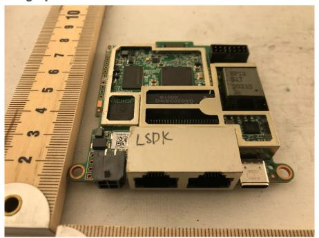
**Photograph 6: Main PCB Showing Ethernet Ports**
