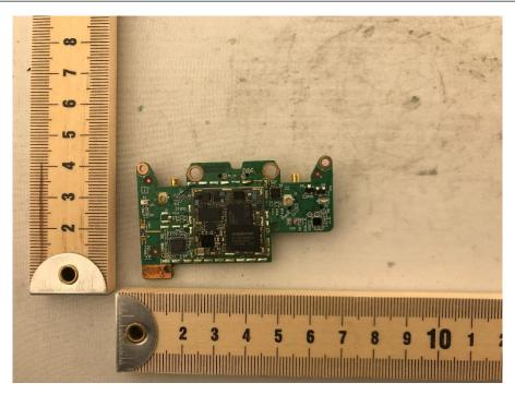
**Photograph 9: Top View of RF PCB**
