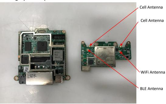
Photograph 4: Top View of DUT With RF Board Removed
