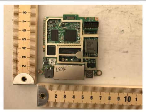
Photograph 7: Top View of Main PCB
