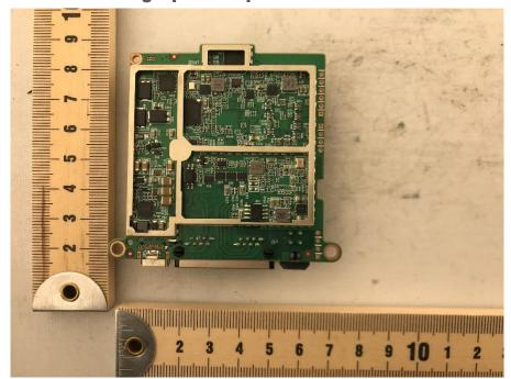
**Photograph 8: Bottom View of Main PCB**
