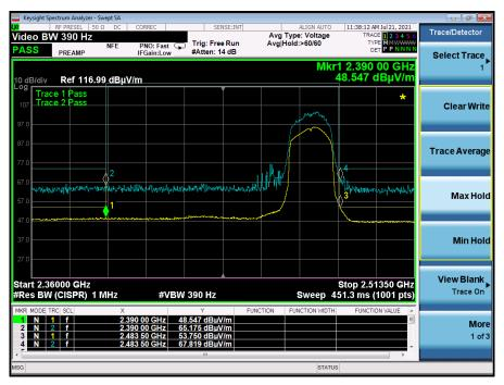
Graph 8: Radiated Higher Band Edge Plot g-Mode – 2472 MHz
