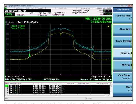
Graph 13: Radiated Middle Band Edge Plot n40-Mode – 2437 MHz
