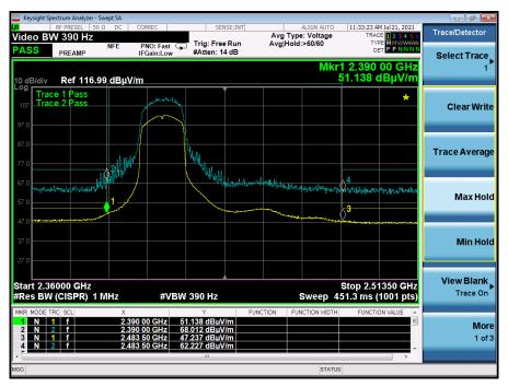
Graph 6: Radiated Lower Band Edge Plot g-Mode – 2412 MHz
