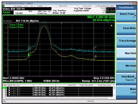
Graph 3: Radiated Lower Band Edge Plot b-Mode – 2412 MHz
