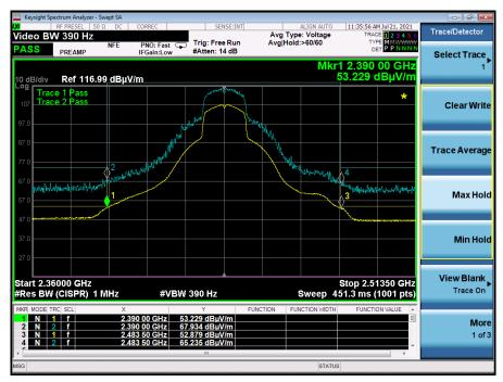
Graph 7: Radiated Middle Band Edge Plot g-Mode - 2437 MHz
