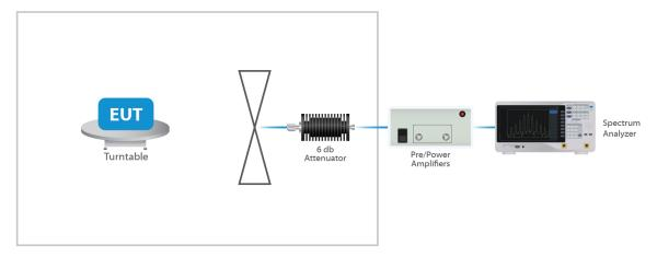
Figure 3: Radiated Emissions Test
