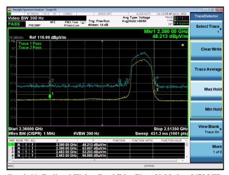
Graph 11: Radiated Higher Band Edge Plot n20-Mode – 2472 MHz
