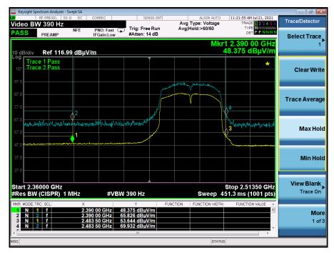
Graph 14: Radiated Higher Band Edge Plot n40-Mode - 2462 MHz
