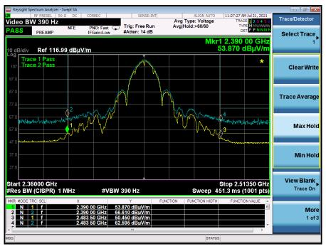
Graph 4: Radiated Middle Band Edge Plot b-Mode - 2437 MHz
