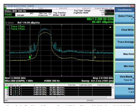
Graph 9: Radiated Lower Band Edge Plot n20-Mode – 2412 MHz
