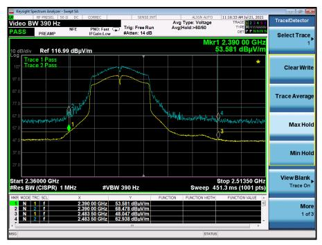
Graph 12: Radiated Lower Band Edge Plot n40-Mode – 2422 MHz
