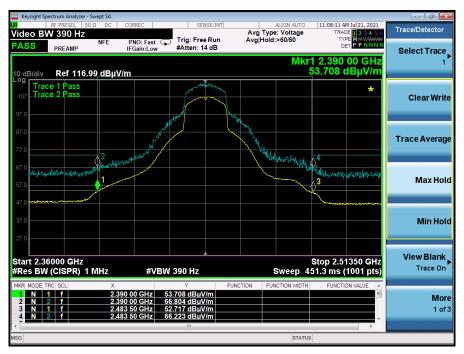
Graph 10: Radiated Middle Band Edge Plot n20-Mode – 2437 MHz
