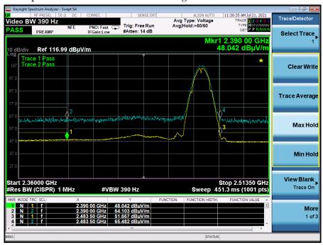
Graph 5: Radiated Higher Band Edge Plot b-Mode - 2472 MHz
