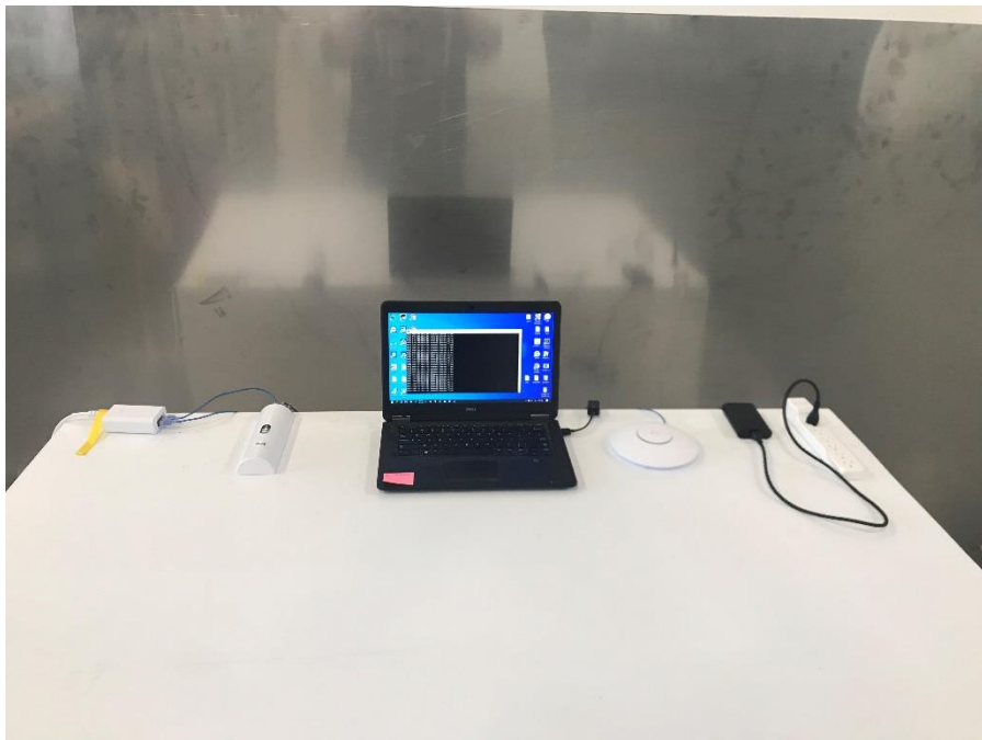
Photograph 4: Front View Test Set Up Conducted Emissions
