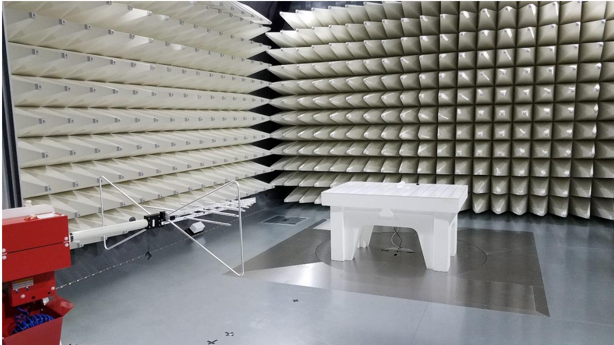
Photograph 1: View Test Set Up Radiated Emissions 30 – 1000 MHz
