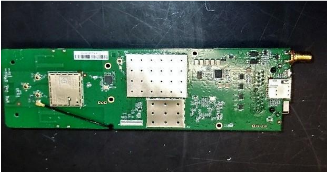
Photograph 4 – Internal Back View of the EUT With RF Shielding
