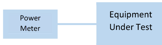
Figure 3: Output Power Measurement
