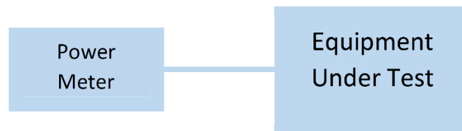
Figure 3: Output Power Measurement
