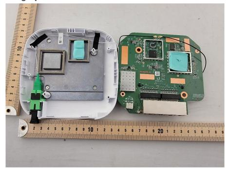
Photograph 2: Back View of Circuit Board and Back Heat Sink
