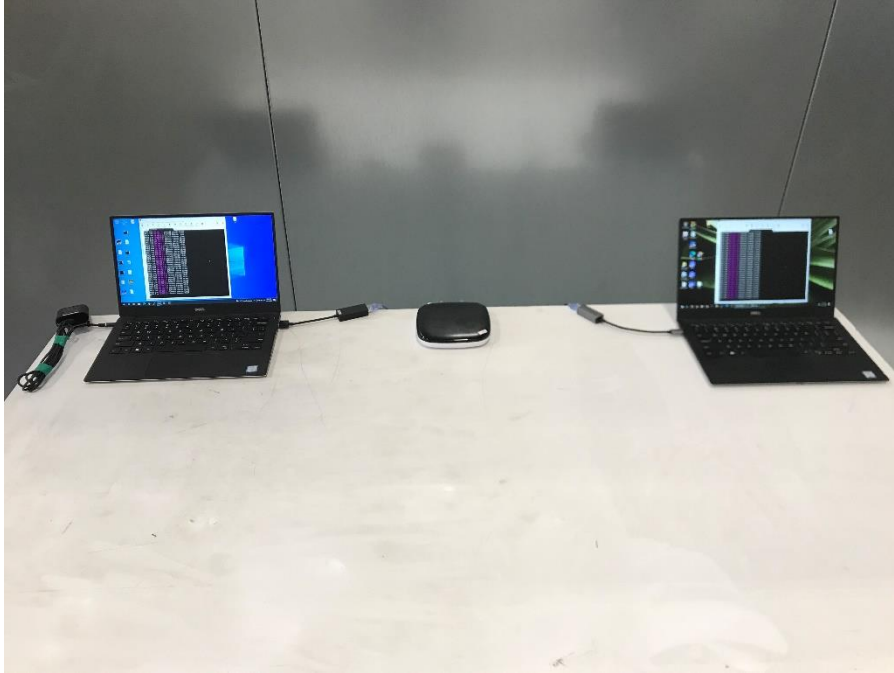
Photograph 4: Front Test Set Up AC Mains Conducted Emissions
