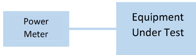
Figure 3: Output Power Measurement
