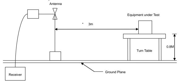
Above 1GHz Test Setup
