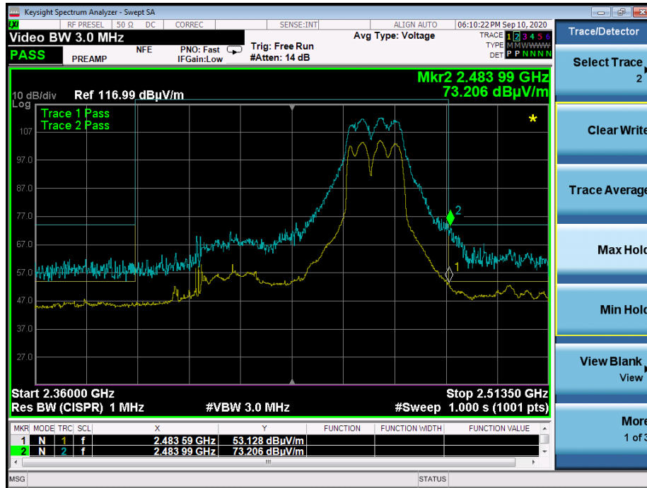
Graph 5: Radiated Upper Band Edge Plot b mode
