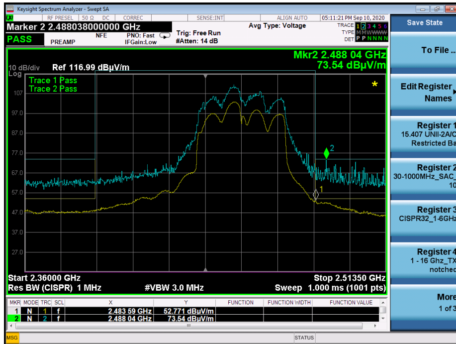
Graph 8: Radiated Upper Band Edge Plot n mode (40)
