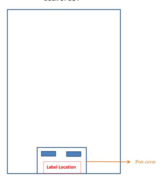
Press down on the center of the port cover and slide it downward to remove it.
