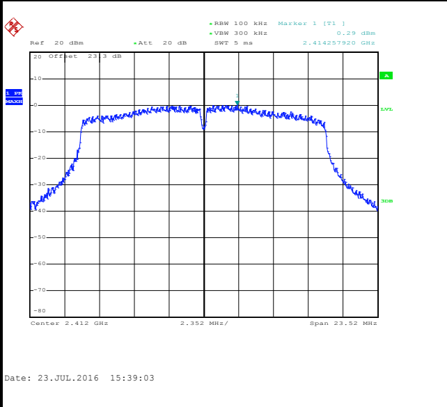
Spurious Emission 30MHz~3GHz
