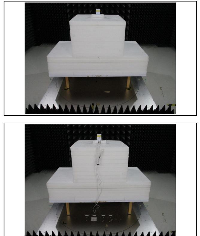
Radiated Emission Above 1GHz Test
