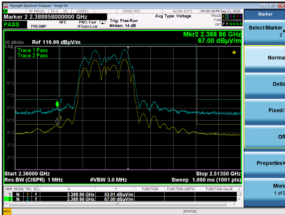
Graph 4: Radiated Lower Band Edge Plot n mode (40)
