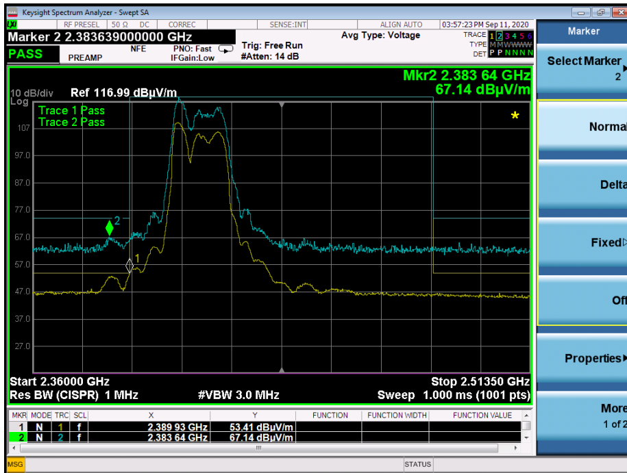
Graph 2: Radiated Lower Band Edge Plot g mode
