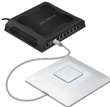
TOUGHSwitch PRO Power Connection Diagram
